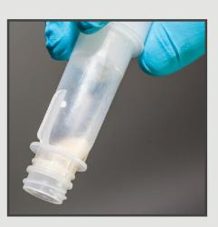
> Shake the tube until a milky solution is obtained.
