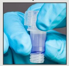
Remove the cap to open the heating tube of the Loopamp™PURE DNA Extraction Kit.
