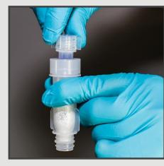
> Screw the heating tube onto the adsorbent tube.
