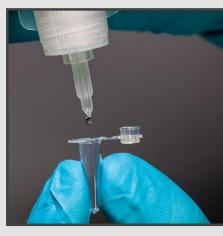
> Extract 30 µl of the DNA directly into the reaction tube by squeezing the adsorbent tube.
