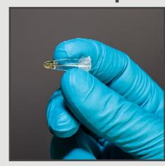
> Mix the contents of the tube by shaking five times.
