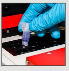
Incubate the tube in the HumaLoop T heating unit for 5 min at 90°C.
