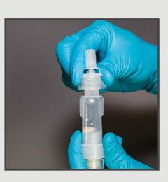
> Screw the injection cap onto the other side of the adsorbent tube.
